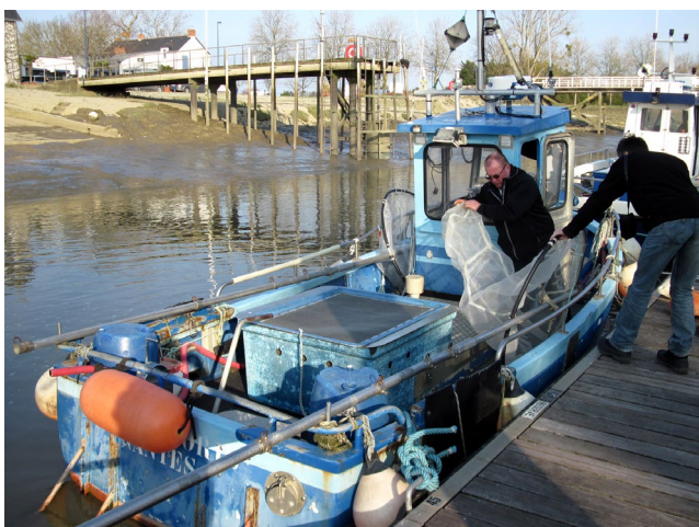
FIGURE 2 Glass eel fishing boat from the Loire River with two push nets attached to the sides and a fish tank with a sieve on top, to store the catch
