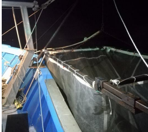
Figure 1. Fishing gear lifted out of water while cod end was emptied.
